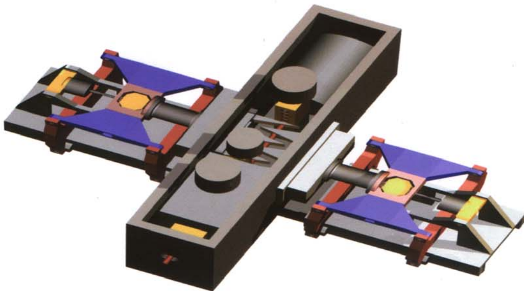
Figure 3: Degrader system with the dual degrader unit that is set-up on a girder. The beam enters the vacuum chamber at the front side. Schematically shown are the diagnostics box, the beam stopper-Faraday cup, the set of retractable scatter foils, the degrader unit, the adjustable set of collimators and the collimator to stop the beam halo.
